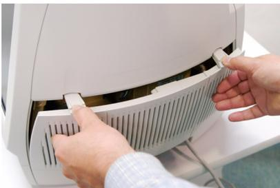
*Figure 9-1 Removing rear cover*
