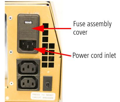
*Figure 9-3 Computer tray fully out, giving access to fuse assembly*
