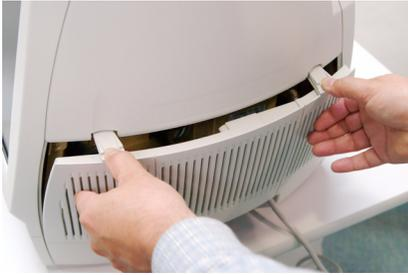
Figure 1-4 Removing rear cover
